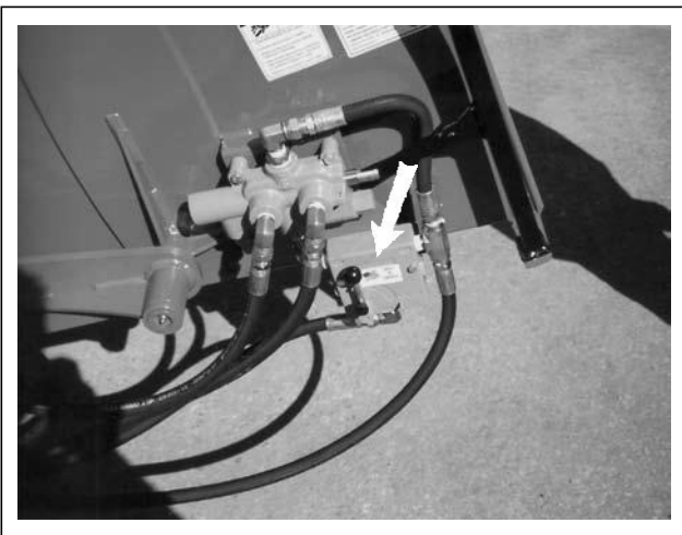
Fig. 22 FLOW CONTROL VALVE
